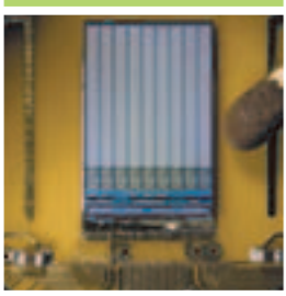
Pixel Matrix with 18 x 160 pixel cells. For comparison a part of a match is shown.
