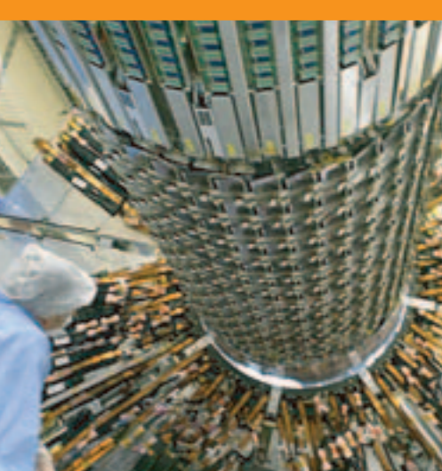
Assembling the ATLAS SemiConductor Tracker (SCT) which consists of approximately 16 000 silicon microstrip detectors with 6.3 million readout channels, built into 4 088 modules
